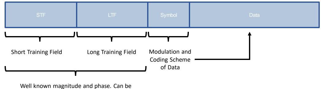
Well known magnitude and phase. Can be used to get start of the packet + **equalization**
