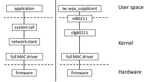
Flow of data (left) and management/configuration (right) through the Linux kernel
