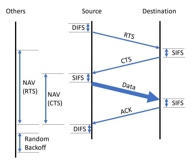
**DCF**: Distributed **Coordination Function DIFS**: DCF Interframe Space **SIFS**: Short Interframe Space **RTS**: Request To Send **CTS**: Clear To Send **ACK**: Acknowledgement **NAV:** Network Allocation Vector
